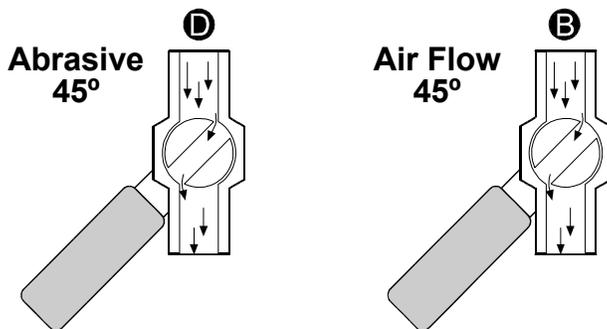
Set Air Flow Valve (B) approximately half way open or at 45° angle. Adjustments will need to be made as wear occurs to Blast Hose (K) and Blast Nozzle (T).
