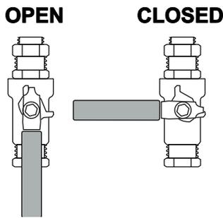
**3.1 Pressure Pot Settings:** The Pressure Pot has two adjustment ball valves that can regulate the abrasive/air flow mixture. The standard settings for the pressure pot should be made as follows:
